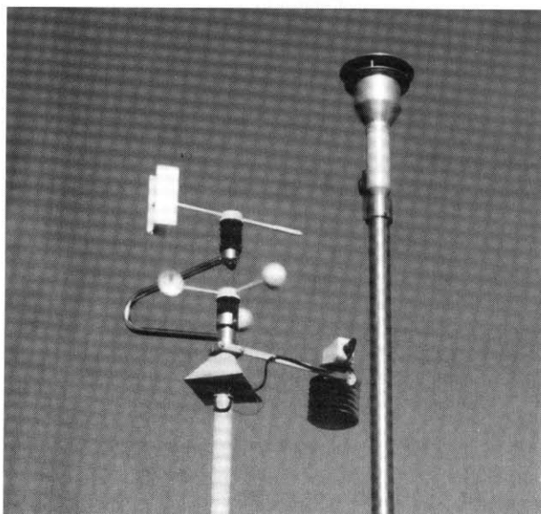
Figure 1.3. A station for monitoring air pollutants. Photo: L. Rydén.
