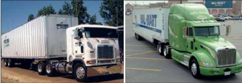
Figure 11.5. Standard truck and an energy efficient truck, the Eaton/Peterbilt Diesel-Assist Hybrid. Source: http://www.naturaledgeproject.net/factor5.aspx
