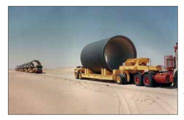
Figure 11.3. The transport of pipe segments for the Great Manmade River in the Sahara desert, Libya: a network of pipes that supplies water from the Nubian Sandstone Aquifer System, (Photo: Jaap Berk, The Netherlands, https://commons. wikimedia.org/w/index. php?curid=12200100
