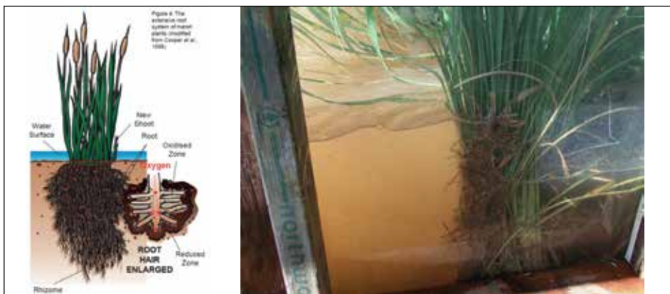
Figure 7.7. Oxygen transport for the root zone (left) and filtering effect of sedge (right) (Wetlands International, 2003).
