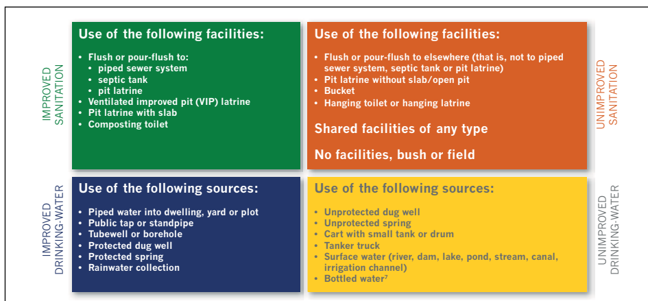
Figure 2.2 Unimproved and improved drinking-water and sanitation facilities. Source: Progress on Sanitation and Drinking Water. 2010 UPDATE. http://www.unicef.org/eapro/JMP-2010Final.pdf
