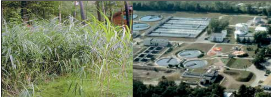
Figure 4.5. Natural (left) and conventional (right) wastewater treatment system
