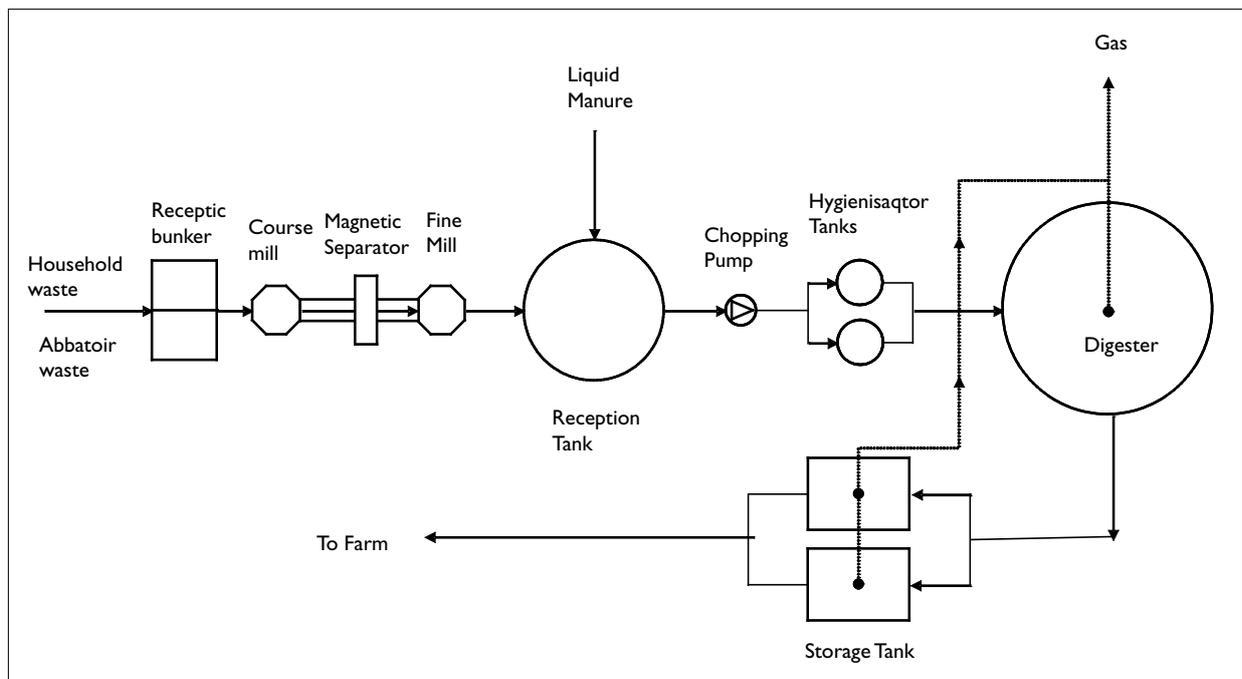
Figure 1. Example of a principle flow diagram for a biogas plant.
