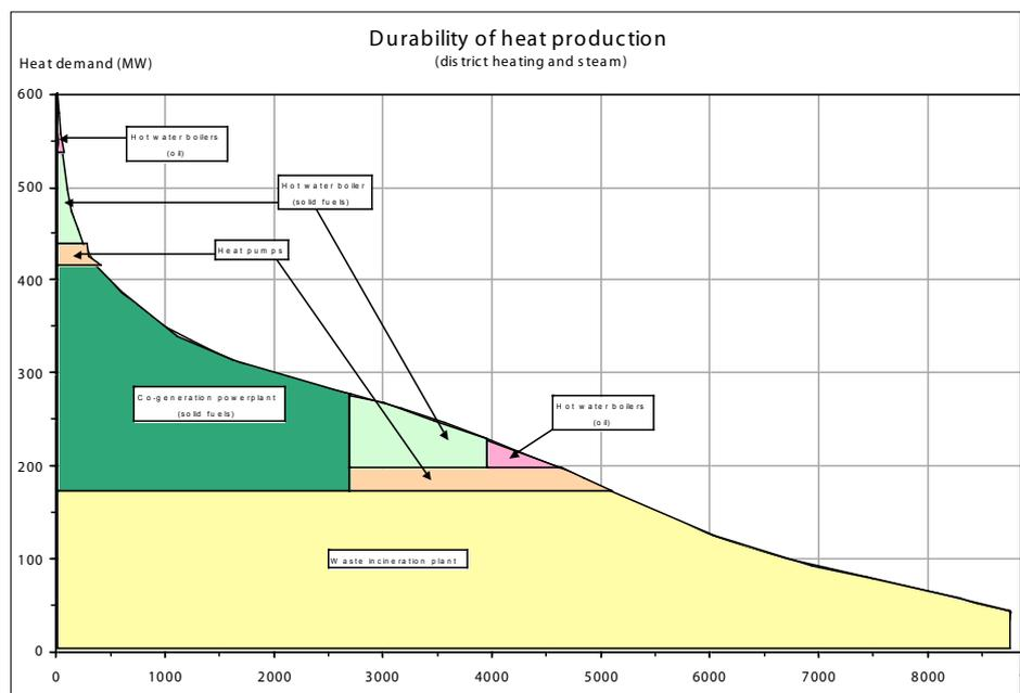
Figure 2. Durability of heat production.
