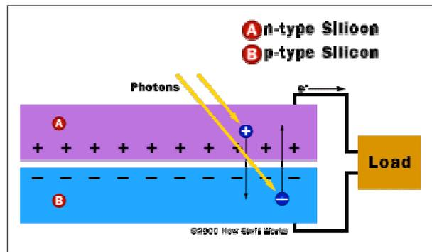
Figure 2 . Operation of a photovoltaic (PV) cell
