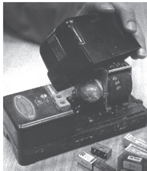
The replacement of the old, rather large, electric relay, containing considerable amounts of mercury, with modern devices illustrates several management principles: dematerialization by using a smaller size, substitution of a harmful material for a less harmful one, and the need for less current when the modern relay is used.
