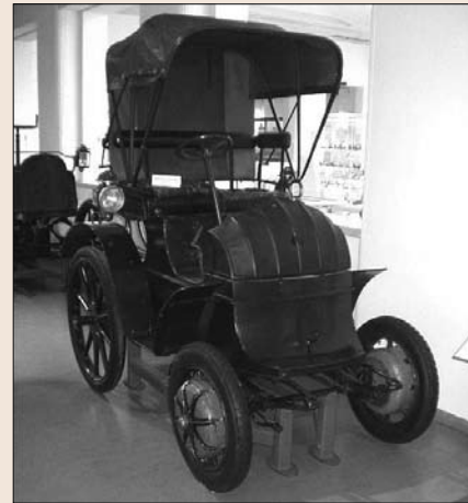
Figure 2.7 The Lohner-Porsche. The electric engine was placed in the front hubs. (The Lohner-Porsche Electric-Car is part of the Exhibitions of the Technisches Museum Wien.)
