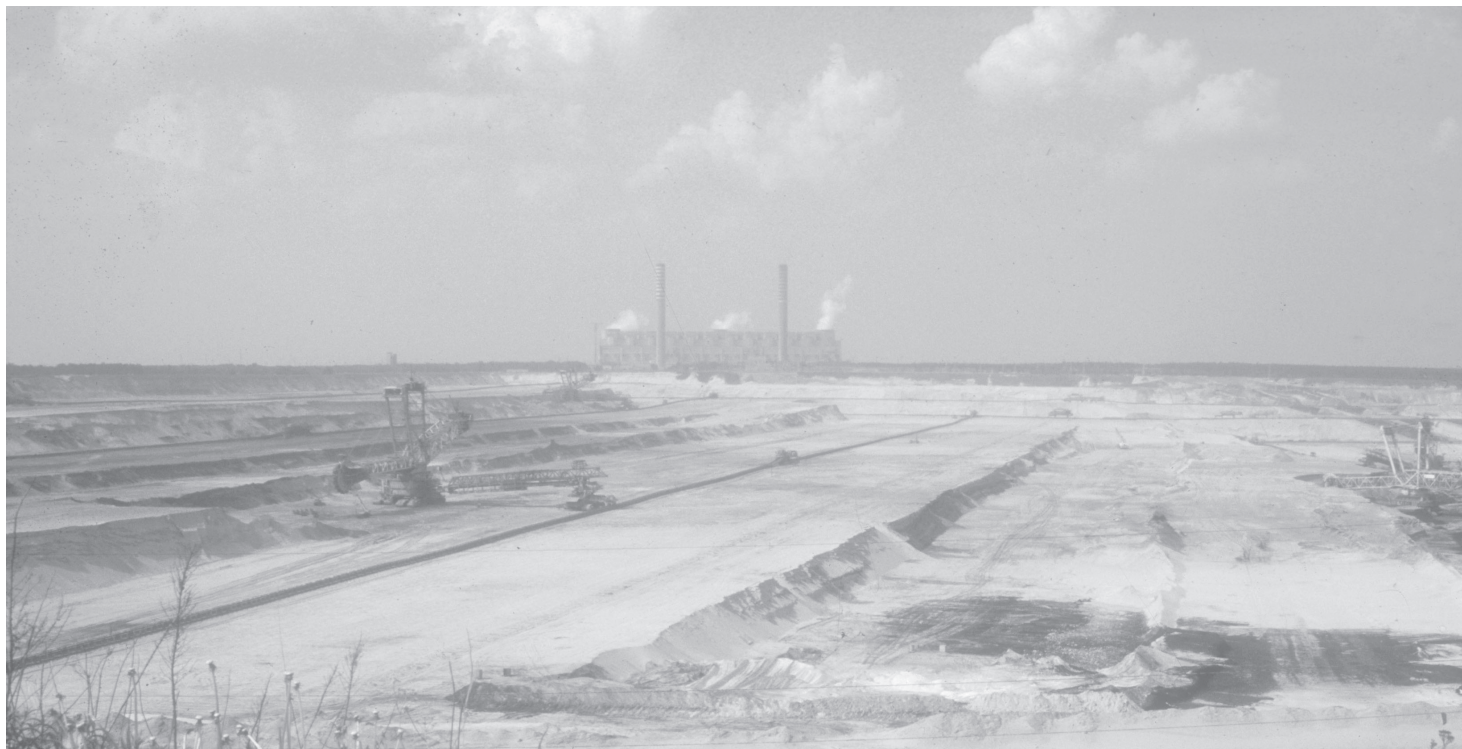
Figure 12.3. Strip mining of brown coal or lignite at Belchatow, central Poland. Coal is one of the main sources of metal pollution, as the metals in the coal, e.g. cadmium and mercury, is emitted during combustion. The Belchatow power plant, seen in the background, is the largest brown coal powered plant in Europe. (Photo: André Maslennikov.)
