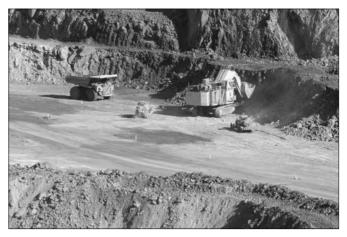
Figure 3.5 Iron and metal mining. *Heavy equipment digs and hauls ore inside an enormus open pit mine. (Photo:iStockphoto)*
