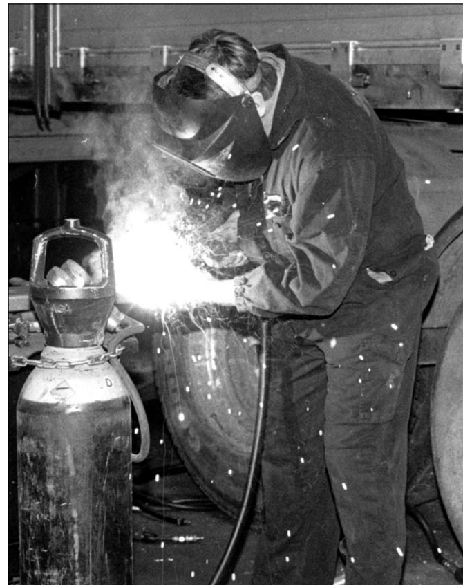
Figure 9.3 The work environment of a welder has to be properly arranged to be safe. Risk assessment relates to e.g. fire, temperature, intense light, and possible leakage of the gases used for the welding. Photo: Inga-May Lehman Nâdin.
