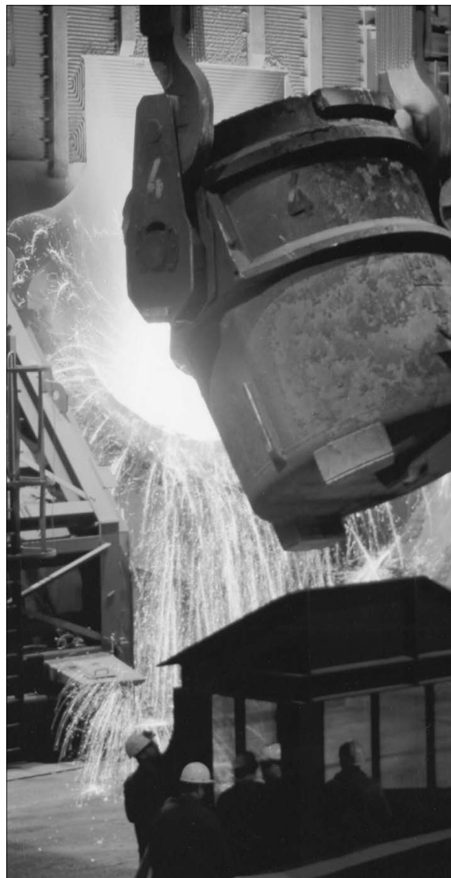
Figure 2.1 Converter. Steel is melted from such raw materials as pig iron, scrap and alloy additions. Photo: Stahl-Zentrum.
