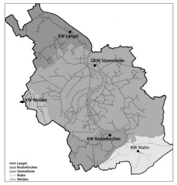
**Figure 3.1 Wastewater Treatment area of Cologne StEB.** *The area served by the company is about 405 km<sup>2</sup>. The five wastewater treatment plants are, from top, KW Langel, Stammheim, Weiden, Rodenkirchen and Wahn. A special challenge is the high amount of water protection areas (about 46%), which make the treatment of wastewater more difficult.*
