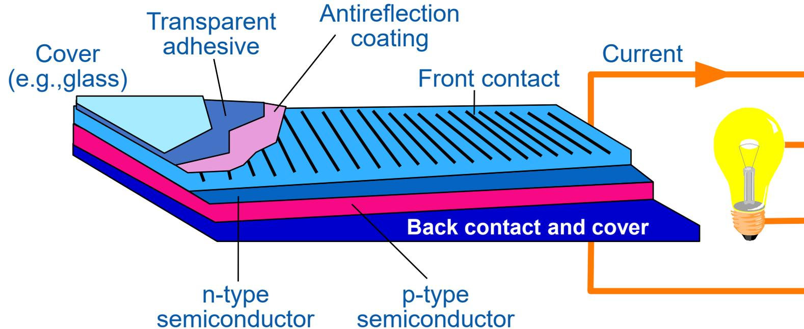
$$\text{Solar cell efficiency (\%)} = \frac{\text{Power out (W)} \times 100\%}{\text{Area (m}^2\text{)} \times 1000 \text{ W/m}^2}$$
