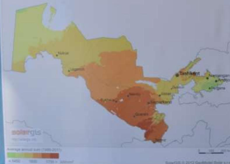
North-West(Nukus): 1500 kW-h/kW peak for fixed inclination, 1700-1800 kW-h/kW peak for one-axis tracking device
