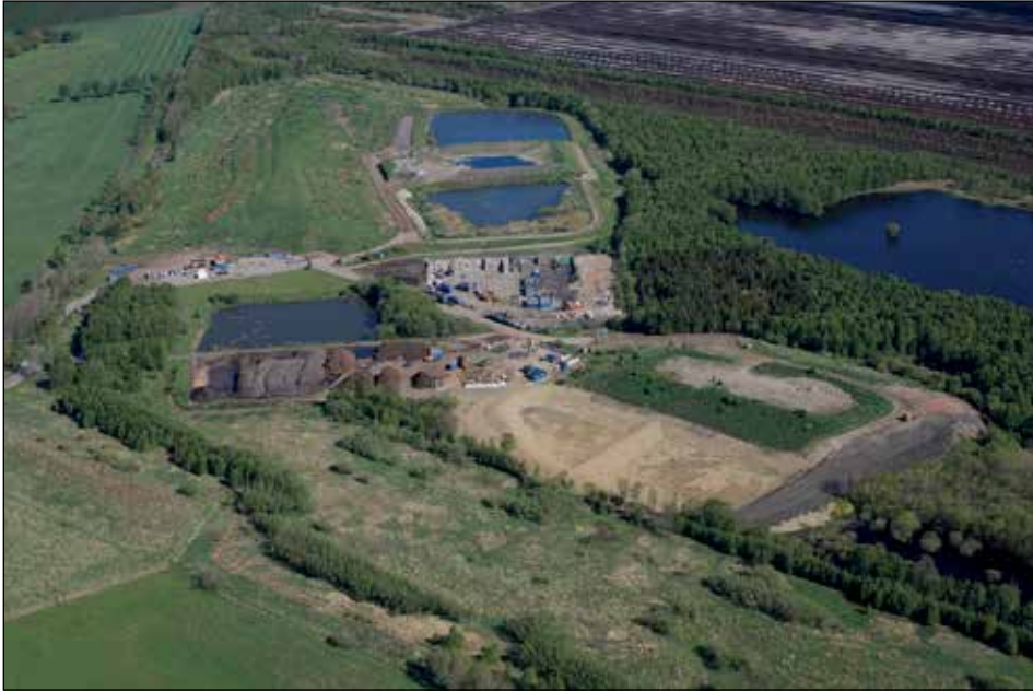
Figure 10.4 A landfill in Rönneholm, the south of Sweden. The landfill is still operating, but some pits have already been closed and reclaimed. On the left there is a reservoir for leachate collection and treatment.
