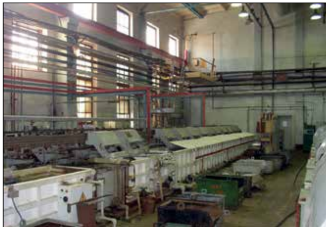
Figure 17.2 Applying protective or decorative coatings using the electro-chemical method produces hazardous compounds based as a rule on heavy metals causing serious environmental problems and great difficulties during the precipitation disposal.
