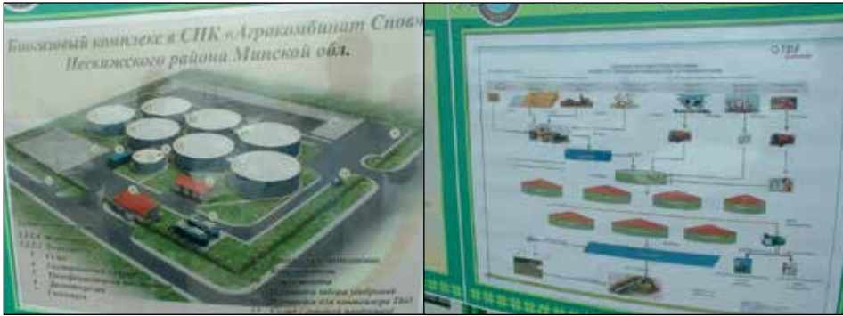
Figure 16.5 The scheme of a biogas complex in the agricultural complex “Snou”, Belarus, electric capacity is 2,1 MWt.
