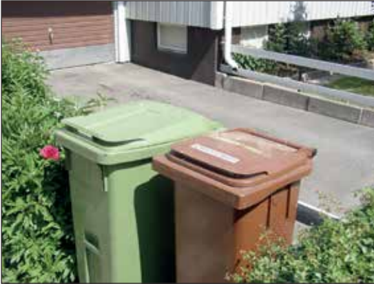
Figure 12.2 An example of a flat-by-flat scheme of waste collection in Uppsala, Sweden. The house owner placed two mobile containers at the side of the road. One container is filled with waste going to the incineration plant; the second containing biodegradable waste is going to be used for the production of compost or biogas.
