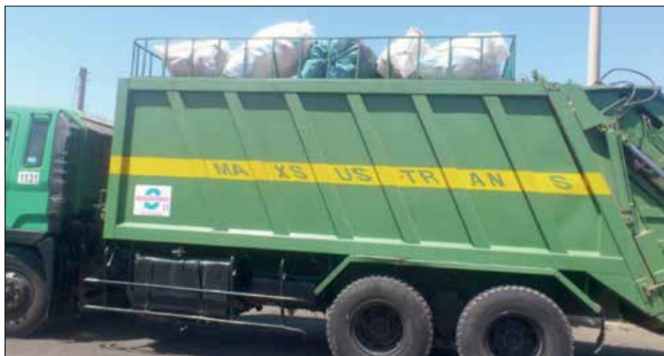
Figure 12.6 A garbage truck in Tashkent equipped with a roof rack for paper and plastic waste. Photo: “Makhsustrans”.
