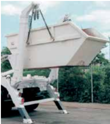
Mounting a shipping container for waste on a truck's chassis
