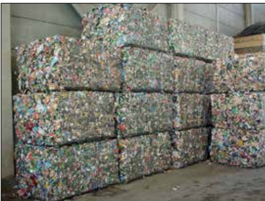
Figure 15.8 Used aluminium cans compressed and prepared for remelting.
