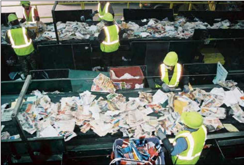
Figure 12.1 Sorting line for paper waste at the waste sorting facility. Paper sorted by type will later be pressed into bales and sent for recycling.
