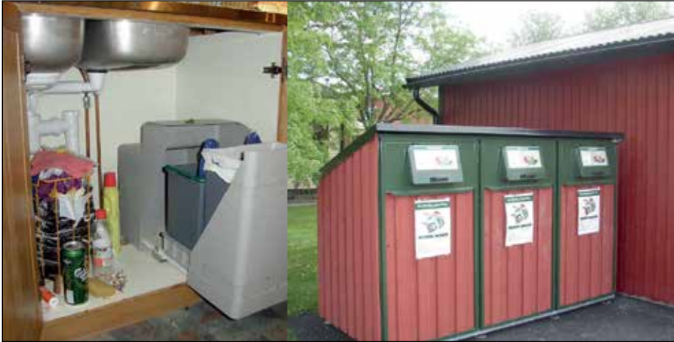
Figure 15.1 Separate collection of waste in a residential sector in Uppsala (Sweden). Separation of waste into fractions (organic waste, plastic, paper and cardboard, glass, metal) starts in the kitchen and is done with simple accumulation containers devices. Large containers for separate collection of garbage are placed near houses
