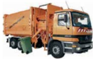
Side-loaded waste truck
