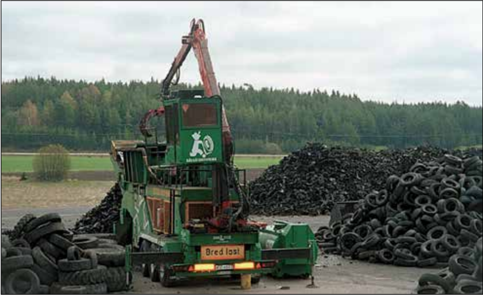
Figure 15.9 Disposal of tyres on a mobile shredding facility on a MSW landfill in Sweden.
