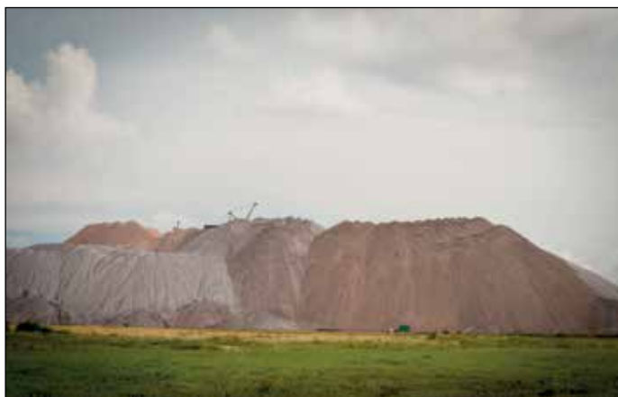
Figure 17.4 Huge volumes of waste are generated during the mining and processing of sylvinitic ore used to produce potassium chloride that is a mineral fertilizer used in agriculture. The picture shows “mountains” of waste near the town of Soligorsk, Belarus, untypical for the local landscape. This waste gravely affects the environment in the region.
